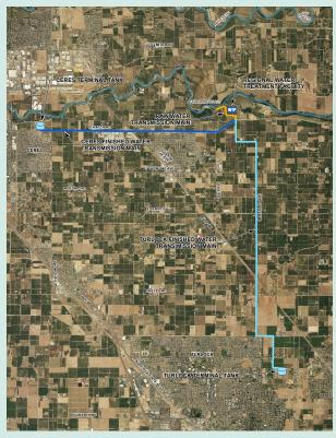
The RSWSP is a collaborative effort that will provide water from the Tuolumne River via an existing set of perforated pipelines installed in gravel about 8-feet below the bottom of the river bed, a new intake structure and pump station, treat the raw water to drinking water standards, and deliver it to the SRWA service areas for municipal and industrial uses. TID will also use the raw water facilities to deliver irrigation water to agricultural users.
